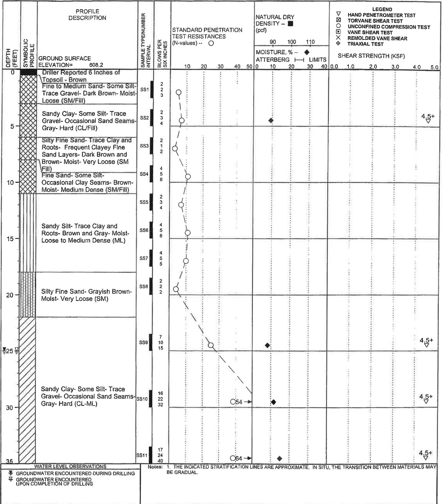
DRILLER: KA      DRILL METHOD: Hollow-Stem Augers      WATER LEVEL DURING DRILLING: 25'      WATER LEVEL      HOURS AFTER COMPLETION:
