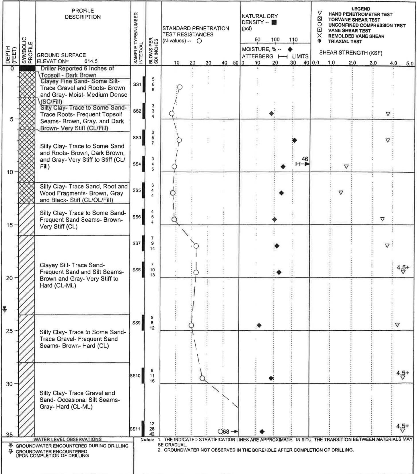
DRILLER: KA      DRILL METHOD: Hollow-Stem Augers      WATER LEVEL DURING DRILLING: 23'      WATER LEVEL      HOURS AFTER COMPLETION:
