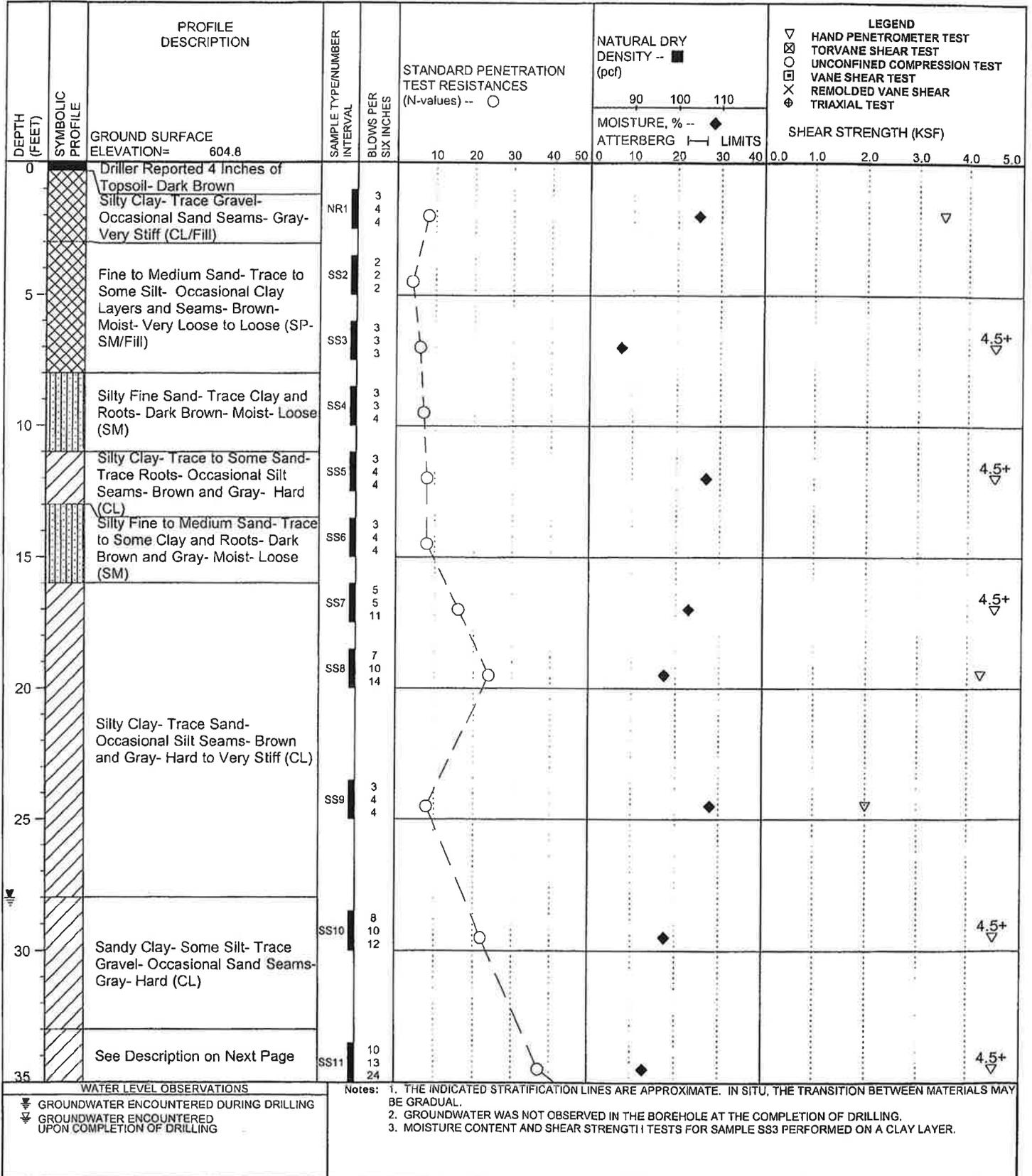
DRILLER: KA      DRILL METHOD: Hollow-Stem Augers      WATER LEVEL DURING DRILLING: 28'      WATER LEVEL      HOURS AFTER COMPLETION:
