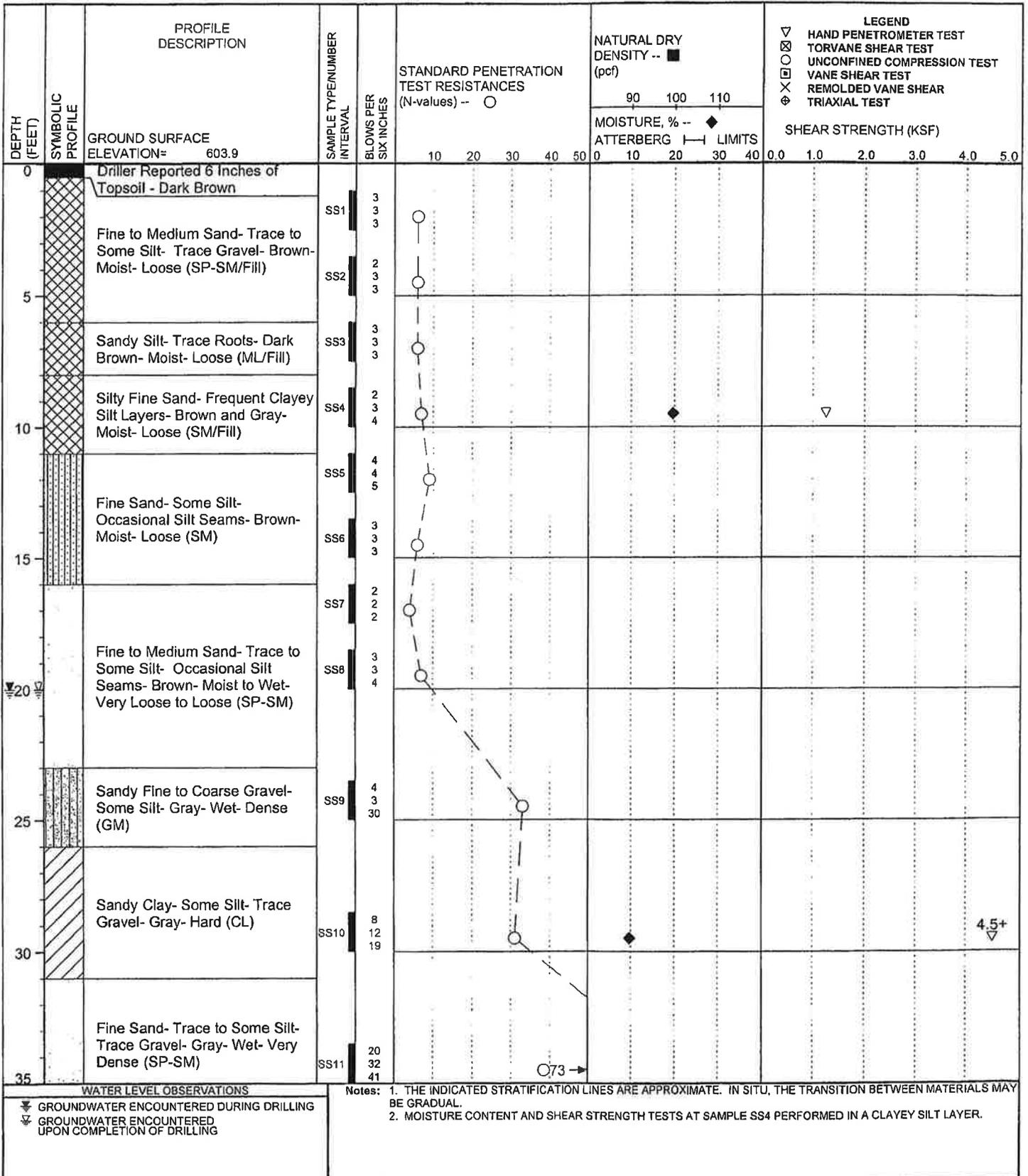
DRILLER: KA DRILL METHOD: Hollow-Stem Augers WATER LEVEL DURING DRILLING: 20' WATER LEVEL HOURS AFTER COMPLETION:
