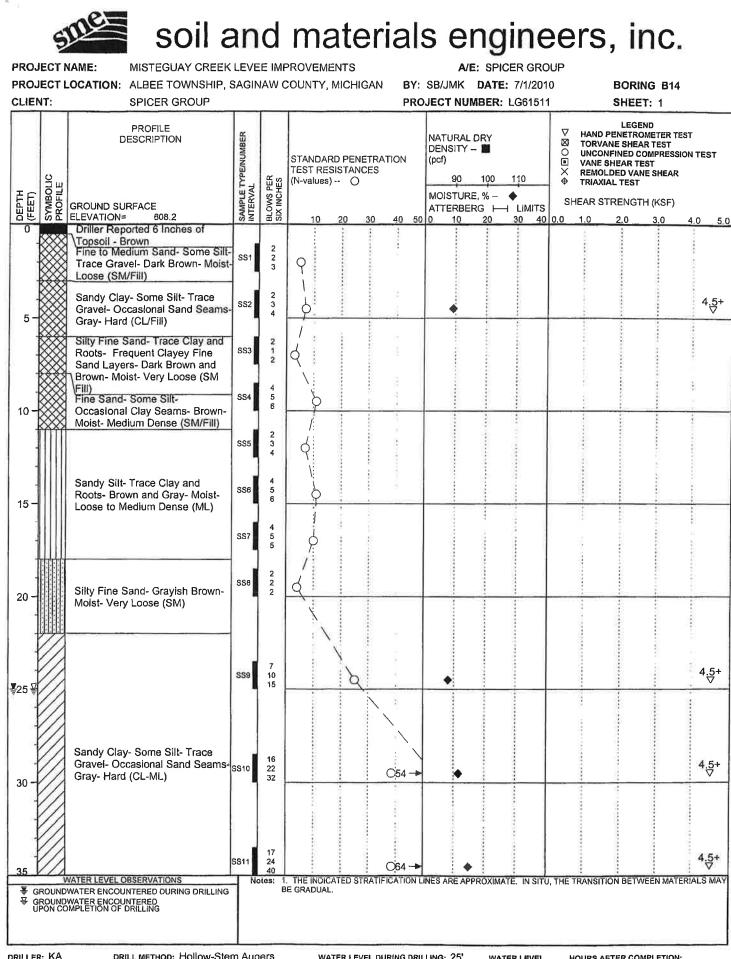
DRILL METHOD: Hollow-Stem Augers BACKFILL METHOD: Bentonite Chips WATER LEVEL DURING DRILLING: 25 WATER LEVEL UPON COMPLETION: 25'
